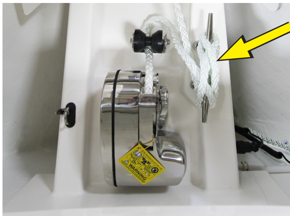
Windlass and anchor rode cleat (typical)
