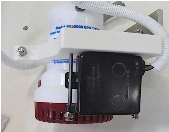
Typical bilge pump and float switch (right)
