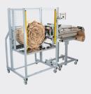
The Coiler is a bolt-on solution designed to be used in conjunction with the Packmaster™ Pro system in order to automate the process of producing consistent, large quantities of highly protective paper coil.
