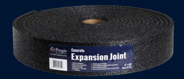
Pregis Concrete Expansion Joint is an essential component used in concrete construction to manage the natural movement of concrete caused by temperature changes, moisture, and ground shifts. Made from polyethylene, the Joint creates intentional gaps between concrete slabs, allowing them to expand and contract without cracking or causing structural damage.
