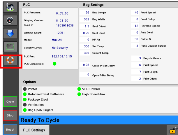
Figure 2-3A. PLC Settings Screen
