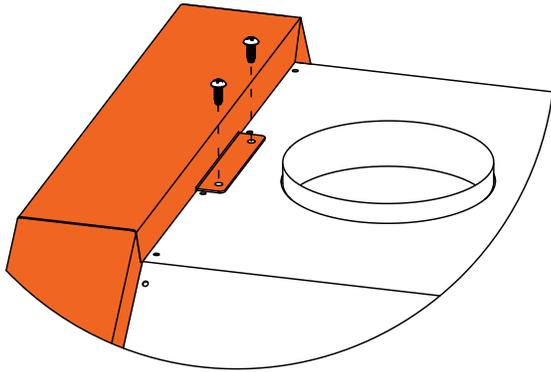
9. Re-install the flue collar on top of the oven with 4 screws, then install the chimney tube.
