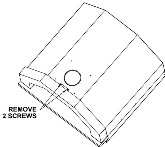
4. Remove the fasteners shown below.
