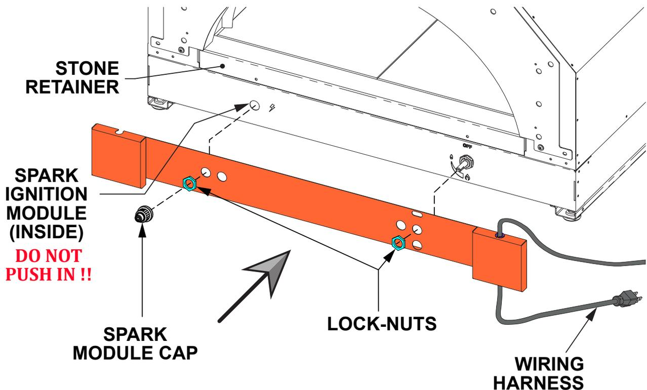
Note: If you mistakenly push the spark module inside the oven, you will need to remove the stone retainer, ceramic pizza stones, and stone supports to gain access.
