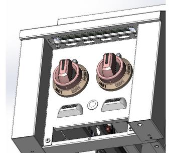
2. The Side burner only has a switch attached to the panel. Follow the same procedure to remove and replace the switch, valve markers, and position markers as seen in the previous section for the Grill.
