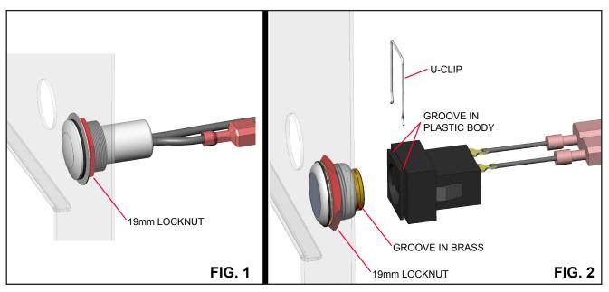
3. With everything reinstalled on your new control panel, you may now reattach the various wire connectors and reinstall the panel to the unit. Be sure you attached the correct wires to the correct switch (Lighting / Rotiss Motor).
