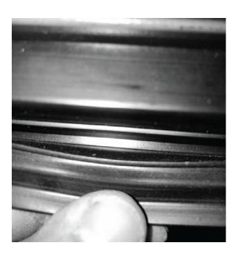
STEP 11 With the door closed, verify the gasket is completely sealing around the cabinet frame.
