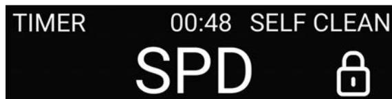
4. Once self clean has completed, an audible alert will sound, the timer will show 00:00 and "COOLING" will be displayed. The oven is now in cool-down mode. See table for times.
