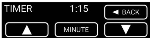
5. The timer has been set and displays the amount of time remaining. The timer counts down in 1 minute increments.
