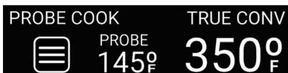
5. Once PROBE COOK has reached the set temperature, the heating elements will shut off. An audible alert will sound a total of 3 times at 1 minute intervals, or until the user cancels the alert and is prompted to turn both control knobs to OFF.
