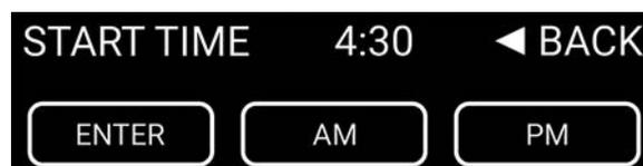
7. The display will revert back to the default display showing the delayed start time. It shows cooking will start at 4:30PM.
