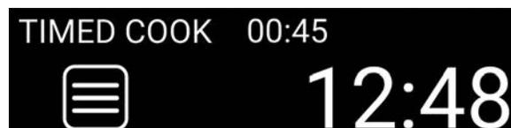
7. Once TIMED COOK has ended, an audible alert will sound a total of 3 times at 1 minute intervals, or until the user cancels the alert and is prompted to turn both control knobs to OFF.
