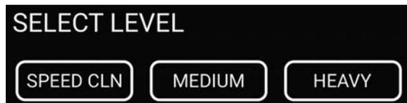
3. Once selected, the display will show "SELF CLEAN" and the selected cleaning level (SPD, MED, or HVY). The door will latch and the lock icon and the time remaining are displayed. The oven cavity will reach a temperature of approx. 825°F [440°C].
