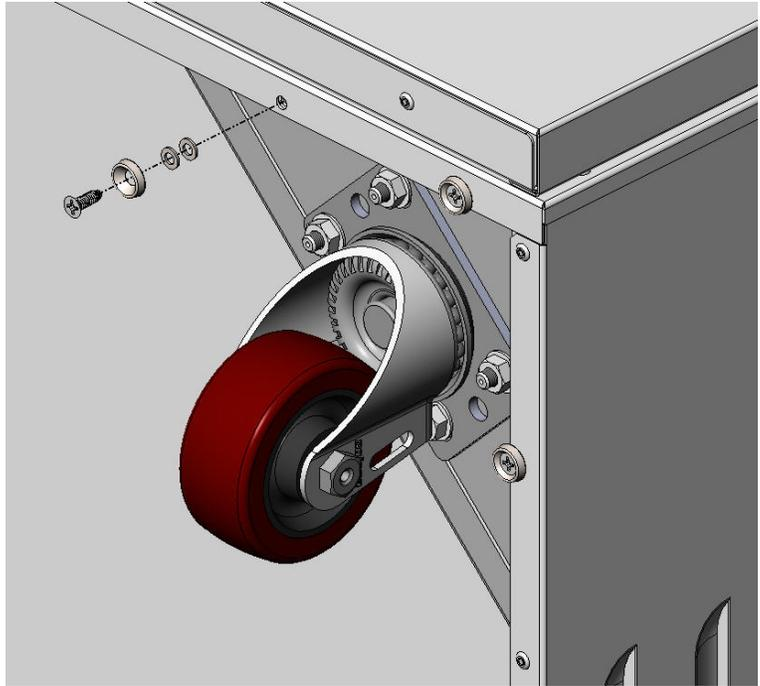
4. Install the caster cover by positioning the keyhole over the screws & washers you installed in Step 3 and slide toward the rear of the cart. Tighten the screws. Repeat for opposite side.
