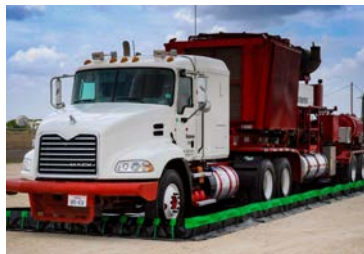
Vehicle Spill Containment
