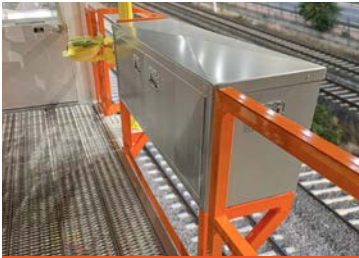
Tool Box for Loading Platforms
