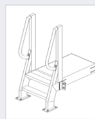
Sample of unsupported configuration, using a ship ladder attached to a 2' x 3' platform
