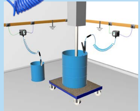
Bond-Rite® Remote Static dissipative GRP enclosure
