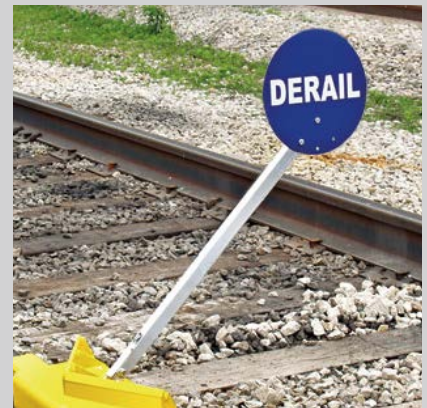
Railcar derail, signs & signals
