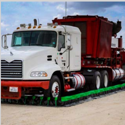
Vehicle spill containment
