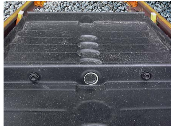
Large, 3"-diameter flow-through channels allow spills to quickly travel from one Pan to the next. Channels are located at the low point in each Center and Side Track Pan.
