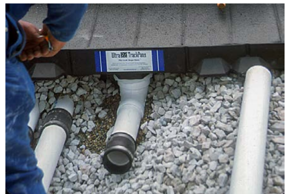
All Center and Side Track Pans are molded with pipe fitting locators at their lowest point. Belowgrade piping can be installed to channel large spills to oil/water separators, holding ponds, etc.
