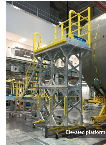
Maintenance and inspection access
