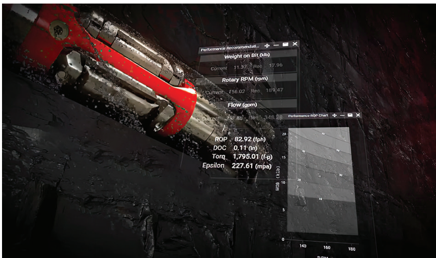
FIG. 3. During an operation in the Middle East, LOGIX drilling performance optimizer indicated that observed degradation in drilling efficiency was due to bit wear/damage. Once the BHA was on surface, the operator confirmed the bit was damaged, as predicted by the algorithm. This solution provided the operator with a reliable decision and reduced rig time.
