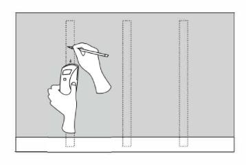
2) Once located, mark the location of the studs where vanity will be fasten too. Use stud finer to located studs.
