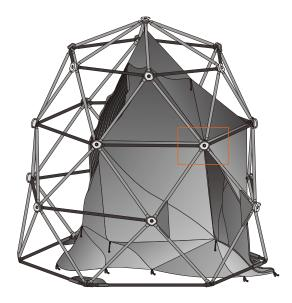
• Locate the green tag. Hang the corresponding bungee over the central hand grip above the door supports.
