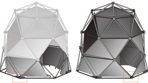
• Attach the five lower bungees to the frame joints around the base of the dome. Then, secure the remaining two bungees to the central frame joint at the base of the door.
