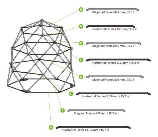
• Lay out the parts as shown but DO NOT take the frames out of their bags. This will slow down the installation process.
