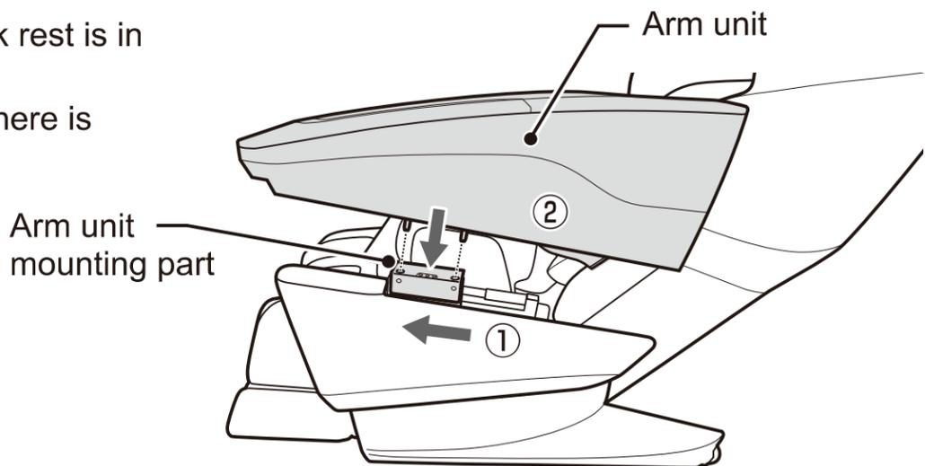
2. Align and close the fastener on the main body backrest and the arm unit one.
