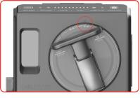
**4.** Position the *lid* so the unlocked arrow icon aligns with the upsidedown arrow on the front of the unit.
