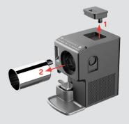
Before disassembly, wait 10 minutes for the cylinder to defrost.
