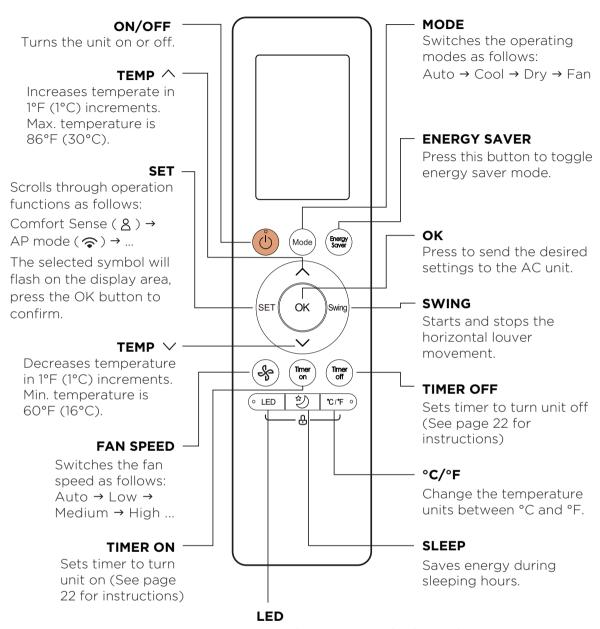
Turn the unit's LED display and control panel beeps on or off.
