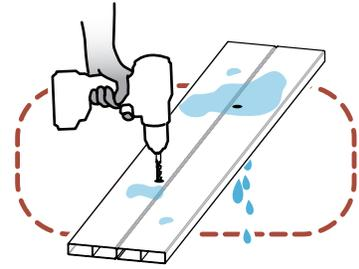
**Note:** For best plant growth, it is recommended to drill (2) 3/4" diameter drainage holes in part (G) roughly 12" apart.
