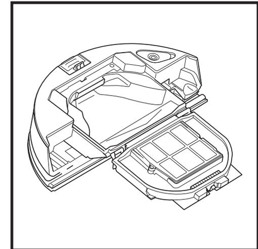
Look between the filter and the plastic shield and make sure there is no debris buildup.
