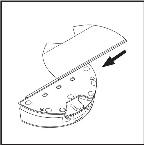
Attach the mopping pad by inserting the flat edge of the pad through the slot in the pad plate on the Vac & Mop 2-in-2 Dust Bin. Pull the mop pad all the way through the slot until it is securely inserted.
