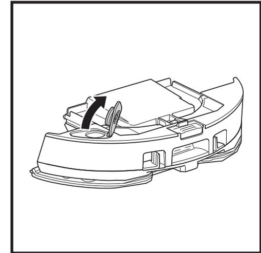
To open the dust bin lid, pinch the side latches in the finger slots and hold them while lifting the lid.
