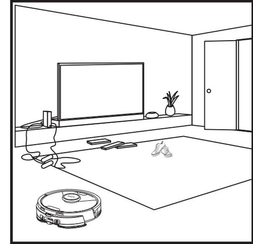
The robot's object detection technology helps it navigate around obstacles taller than 4.5" in height. Clear away small objects that may interfere with the cleaning path of your robot.
