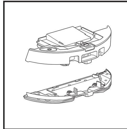
To start vacuum-only cleans, remove the pad plate from the robot dust bin.
