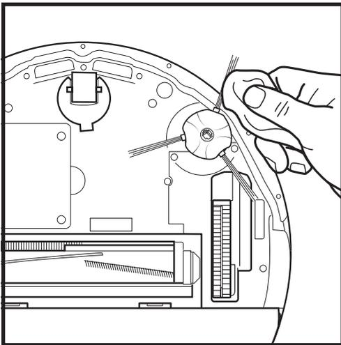
Carefully unwind and remove any string or hair wrapped around the long single side brush.
