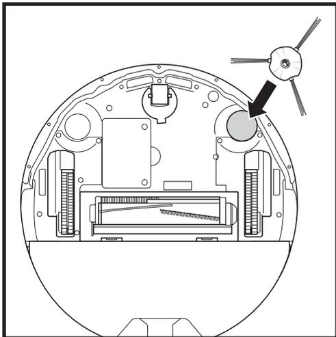
Snap the included long single side brush onto the square peg on the bottom of the robot. The brush will spin clockwise when correctly assembled.
