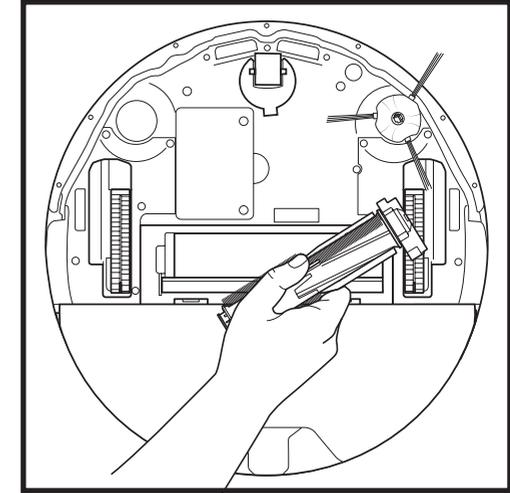
Lift out the brushroll and remove any debris. Remove the end cap to clean out any trapped hair or debris. Replace the end cap once clean.
