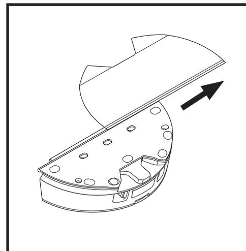
To remove the mopping pad from the Vac & Mop 2-in-1 Dust Bin, detach the pad from the pad plate and slide the pad out of the slot.
