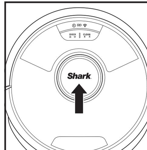
Periodically check the LIDAR navigation module on top of the robot for hair and debris. Gently wipe away any hair or debris from the module.
