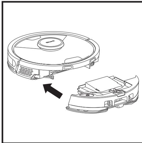
Firmly push the Vac & Mop 2-in-1 Dust Bin into the back of the robot, and ensure both latches click into place. The **CLEAN** button on the robot will illuminate blue when the Vac & Mop 2-in-1 Dust Bin is inserted properly.
