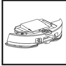
Empty the remaining liquid and the debris from the fluid reservoir after each use. Using a damp cloth, wipe the inside of the dust bin. Let the dust bin air dry for 24 hours before use. DO NOT put Vac & Mop 2-in-1 Dust Bin in the dishwasher.
