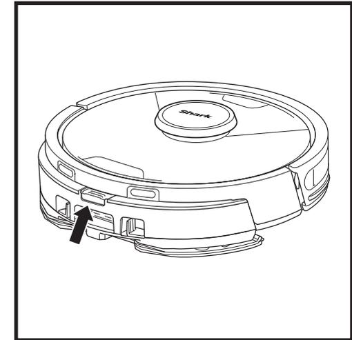
When mopping is complete, remove the Vac & Mop 2-in-1 Dust Bin by pressing the fill port button and sliding it out. The dust bin will auto-evacuate into the self-empty base when the robot docks.
