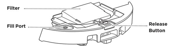
Holds dry debris for vacuuming and water for mopping
