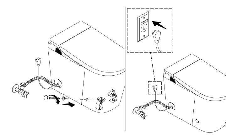
**CAUTION: Risk of product damage.** Do not overtighten the screws. The vitreous shell may chip or break if the screws are overtightened.
