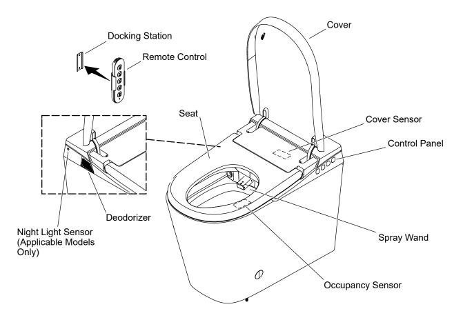
**NOTE:** The toilet cleansing features require an occupant to function. Cover the occupancy sensor area to test the cleansing features.
