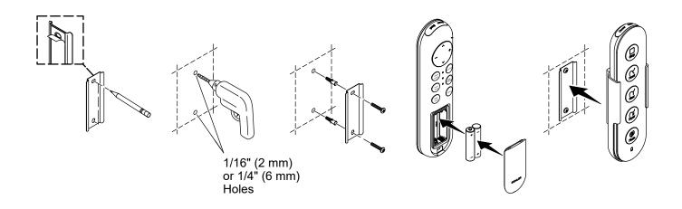
**NOTE:** The double-sided tape on the back of the docking station is only used for prepositioning during installation. For reliable installation, use the screws included in the accessory bag.
