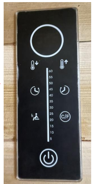
Sauna Control Panel has no Illumination
