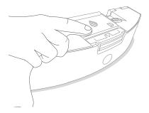
7 Wipe away residue from the undercarriage of the robot. This area must be clear of residue to ensure the dirty water bin slides back into the robot properly.
