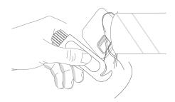
2 Hold the edge clip and pull out the PowerSpin™ Roller Mop.
