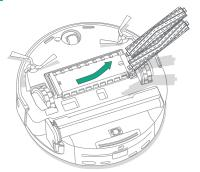
5 Reinstall the multi-surface brush and brush cover in the robot.
