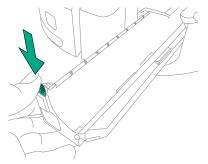
6 Rinse and wipe clean any residue on and from beneath the rubber strip.
