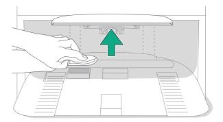
IMPORTANT: When wiping the area clear of debris, be careful not to push debris into the hole located towards the back where air comes out. 2 Reinstall duct vent cover.
