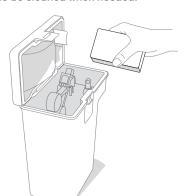
5 Refill the clean water tank with water. Leave the dirty water tank empty.
