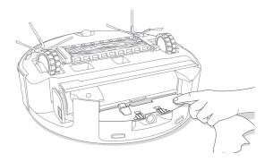
8 Reinsert the dirty water bin back into the robot.
