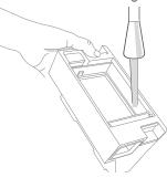
3 Make sure bin is completely dry. Reinsert filter and place bin back in the robot.
