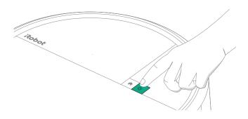
(\*) IMPORTANT: Ensure the latch is properly closed before reinstalling. Failure to properly latch will result in water leakage.
