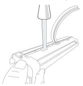
7 Reinsert the rubber strip starting from the same side you pulled to remove the strip marked with an arrow.
