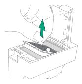
2 Press the dust bin release buttons to remove dust bin.
