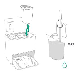
Remove clean water tank (right) from the AutoWash™ Dock. Fill the clean water tank with water
