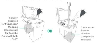
Or, if you do not have the StayClean™ Mopping Concentrate, you may opt to dose the clean water tank with part water, part approved compatible cleaning solution.
