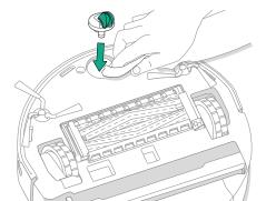
2 Use a flathead screwdriver to pry out the wheel, and remove from the caster.
