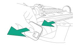
5 Gently peal back the rubber strip by lifting from the corner marked with an arrow, leaving the opposite end attached.
