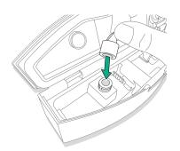
3 Remove black rubber stopper from inside the dirty water bin to clean the inner tubing leading to the drip tray.
