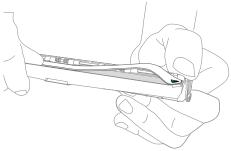
9 With the roller mop cover in the retracted position, clean the actuator so it's free of debris and build-up.
