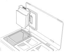
4 Press down on the lid making sure that it is completely closed.
