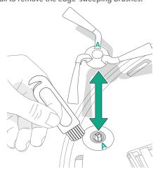
Remove any hair or debris using the cleaning brush, then reinstall the edge-sweeping brushes.
