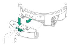
4 Clean out the dirty water bin and tubing by rinsing under water and wiping away the residue.
