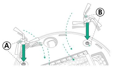
Align the edge-sweeping brush marked with an A to the hardware marked with an A. Press down until you hear a click.
