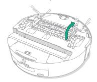
4 Remove any hair or debris that has collected beneath the caps. Replace end caps.
