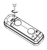
Step 5: Replace cover and tighten screws.
