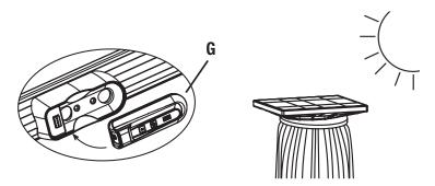
**Step 6:** Remove battery pack (G) from accessories kit and place into the housing located on the arm of the glide handle. Then put the solar umbrella in direct sunlight outdoors to charge the solar panel for 8 hours before the first use.
