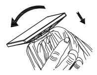
**Step 5:** Put solar panel on top of umbrella and hide the plug and wire inside the cavity at top. Then turn the solar panel clockwise. Do not over tighten.
