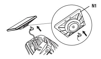
Step 4: Insert plug into socket under solar panel as shown above.
