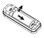
Step 2: Remove cover and remove battery.
