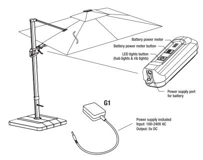
Press the light button once to turn on hub light. Press second and third time to adjust the lighting intensity of hub light. Press fourth time to turn on the rib lights and turn off hub light. Press fifth time to turn on both rib and hub lights. Press sixth time to reach the medium lighting intensity. Press seventh time to reach the most lighting intensity. Press eighth time to turn off all lights.
