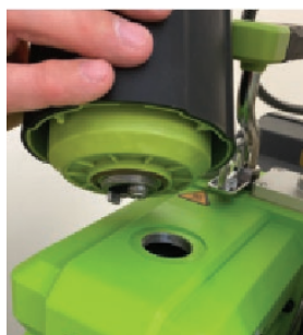
FIGURE 7: Demister removed, showing oil opening
