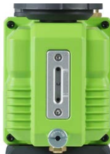
FIGURE 8: Sight glass, showing oil level
