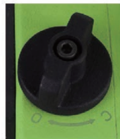
FIGURE 6: Gas ballast shown in "open" position
