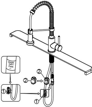
Install the weight clip (E1) at the point of the hose marking "weight here". Insert the weight (E2) onto the clip (E1) by sliding it down onto the clip (E1).
