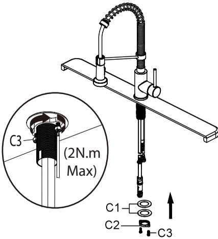
Install the rubber washer and metal washer (C1) onto the threaded mounting shank.
