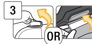
Headrest Style 1: Place Elastic Straps on Headrest Pad Around Headrest/Harness Adjustment Levers Headrest Style 2: Locate Pad Fabric Tab Slot in Headrest
