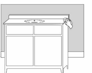
4) Let the assembled vanity sit for 24 hours. Allowing silicone sealant to fully dry. Once dry, proceed to install faucet and drain
