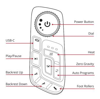
**Power Button** – The power button allows you to turn the chair on and off. Long press the button to turn on/off.
