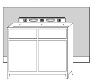
4) Attach your vanity to the wall by screwing through the back of the vanity cabinet. Use the marked stud locations as a guide.
