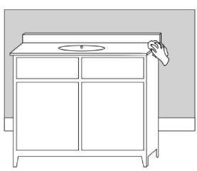
4) Let the assembled vanity sit for 24 hours. Allowing silicone sealant to fully dry. Once dry, proceed to install faucet and drain
