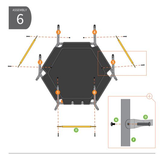
• Fasten the three D short supports to the outside of the F corner frames as shown, using the N large bolts.
