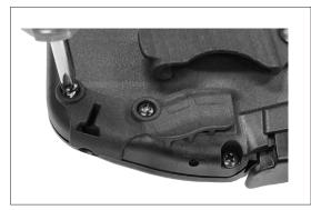
Remove the 2 #6 screws securing the Tuck Device to the holster.
