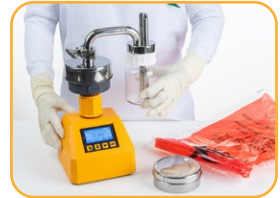
2. Connect the sterile virus system to the aspirating chamber of AIRBIO
