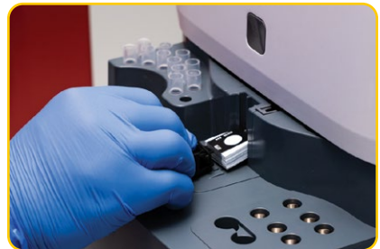
8. The sample is analysed via PCR System
