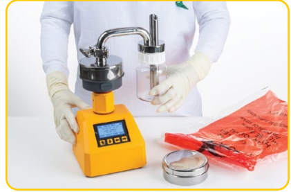
2. Connect the sterile virus system to the aspirating chamber of AIRBIO
