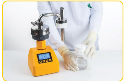
4. Connect the bottle with the collection liquid
