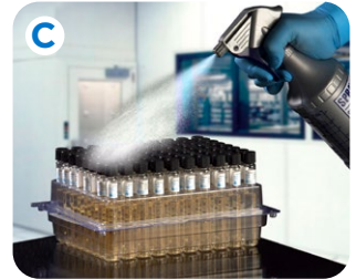
C Spray down entire ReadyRack™ with isopropyl alcohol.
