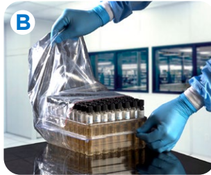
B Take into cleanroom, then remove plastic bag.
