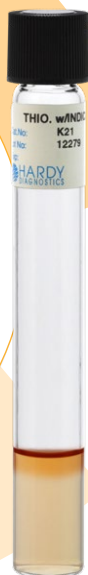
Fluid Thioglycollate Broth Medium (FTM) with Indicator, USP, glass tube, 16x125mm, 10ml fill, Cat. no. K21.
