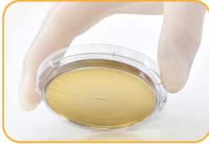
2. Gently press plate to surface without twisting or sliding.
