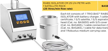
ISOLATOR with battery charger, 1 calibration certificate, 1 S/S satellite, 1 S/S aspirating head (Cat. no. BAS830) with S/S cover head (Cat. no. BAS465), 1 cable connection (5M) (Cat. no. BAS265), 1 cable for data transfer and 1 Robustus medium carrying case.
