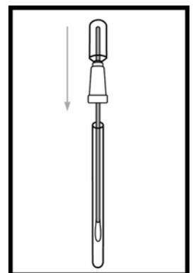
4. Holding the device upright, activate the Ultrasnap by bending the bulb at the top until the plastic Snap-Valve breaks, then bend once more in the opposite direction. Squeeze the bulb twice to expel the liquid-stable reagent contained in the bulb and allow it to flow to the bottom of the tube.
