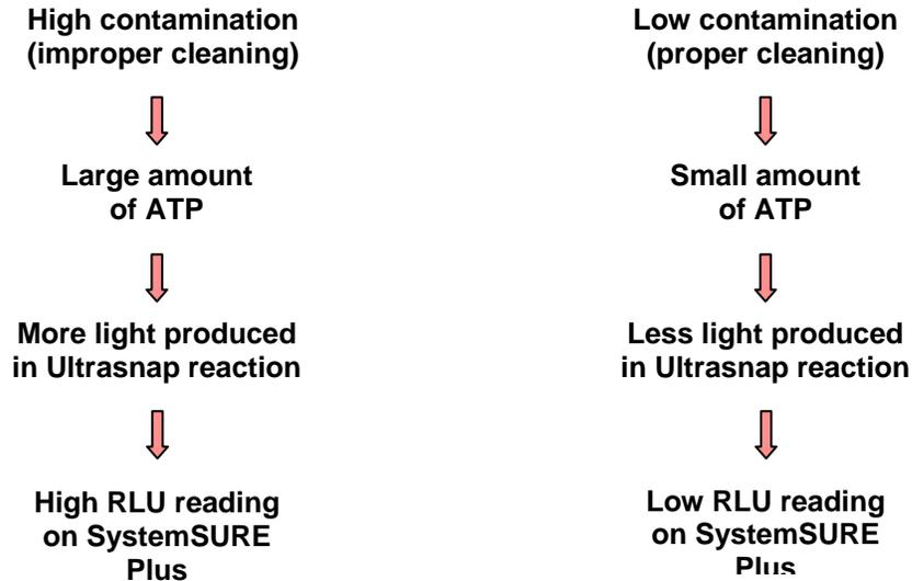
The RLU reading is directly proportional to the amount of ATP collected from the sample. A high RLU reading indicates a large amount of ATP at the test location. This in turn indicates improper cleaning and the presence of contaminants.
