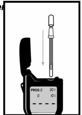
2. Press "OK" on the SystemSURE Plus to initiate measurement of RLU output. Results are displayed on the screen in 15 seconds.
