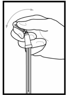
5. Gently shake the device with a side-to-side motion, bathing the swab bud in the liquid-stable reagent. The test is now activated and the bioluminescence reaction is taking place. **For optimal results, the reading should be taken on the SystemSURE Plus luminometer within 5 to 60 seconds of activation.**
