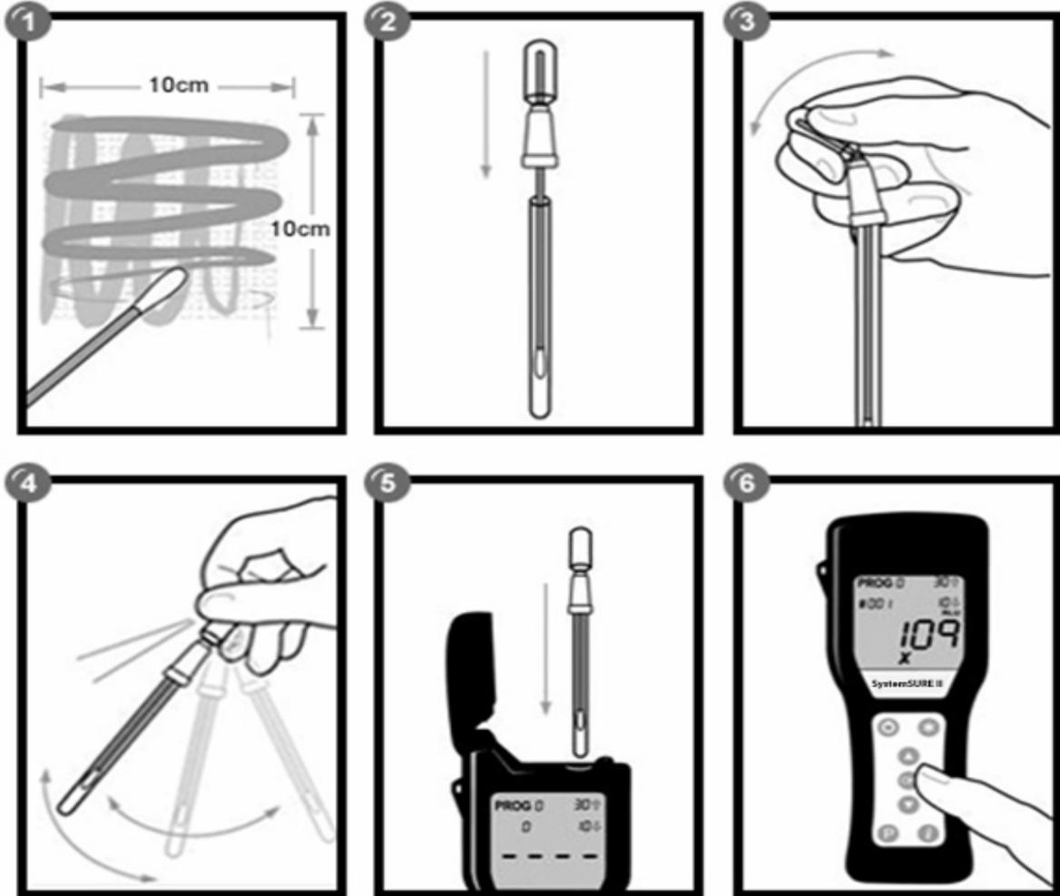
1. Identify the location to be tested and turn on the SystemSURE Plus luminometer. Remove the Ultrasnap swab from the outer tube. Pressing firmly down on the swab tip, collect a sample from a 10 x 10 cm (4 x 4 in) area. Use a side-to-side and up-and-down motion while rotating the swab tip.
