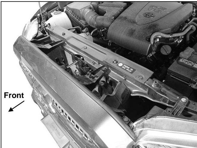
(Fig 7) Remove plastic cover from top of radiator and remove grille
