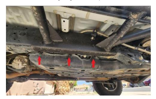
**Step 5.** Position the step slider onto the frame, sliding and aligning the 3 horizontal mounting tabs over the top of the skid plate holes. The slider will naturally mount over the skid plate, then to the frame. When everything is aligned, start to install the supplied hardware in the correct orientation loosely (Bolt, lock washer, then flat washer). Once the slider is on the frame be sure to reattach the parking brake bracket. Then tighten the remaining hardware.
