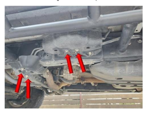
**Step 6.** Remove the two lower bolts holding the KDSS pump bracket. Loosen the long silver bolt on the upper right-hand corner that holds the KDSS pump to the frame. **NOTE: This bolt does not need to be removed completely. It just needs to be loose enough to give the lines enough play to fit the mounting plates behind the lines.**
