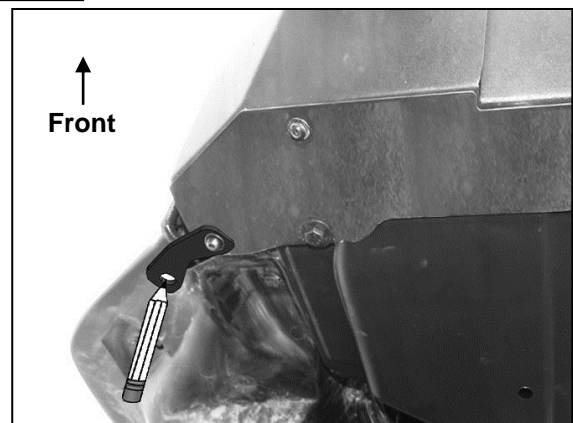
(Fig 25) Mark mounting hole location onto bumper cover. Use 5/16" drill bit to drill hole for mounting hardware (passenger/right side pictured)
