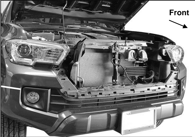
(Fig 8) Grille Removed. Remove factory bumper bolts along the top and bottom of Bumper
