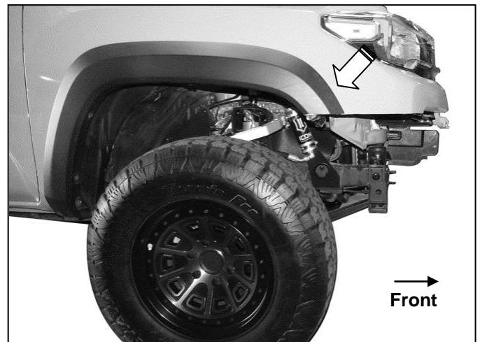
(Fig 17) Reuse the factory fender bolts to attach the front Fender Flares (passenger/right side pictured)
