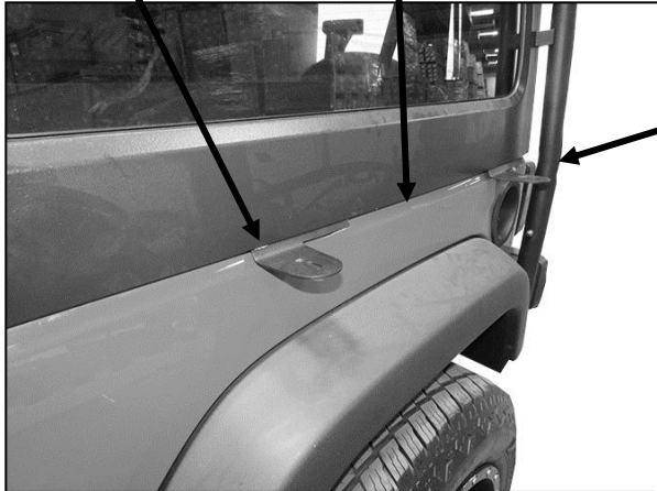
(Fig 9) Reinstall the hardtop and with the driver/left Front, Rear Brackets and Spacer Plates between the top and the body
