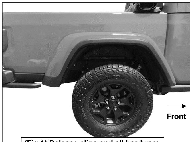
(Fig 1) Release clips and all hardware attaching inner fender liner to outer fender (Passenger/Right side shown)
