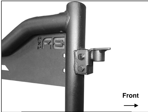
(Fig 6) Driver/left Upper Mounting Bracket attached to back of Door
