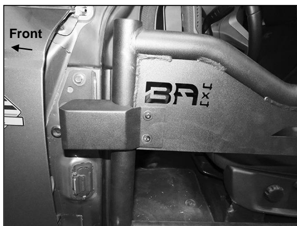
(Fig 16) Attach Upper Hinge Cover to door
