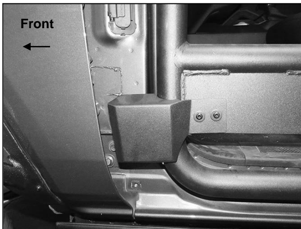
(Fig 18) Attach Lower Hinge Cover to door
