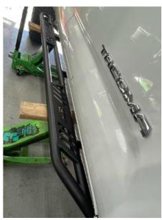
**4.** With a friend or using floor jacks raise the slider to the frame of the truck to test fit and make sure the mounting holes are lined up.
