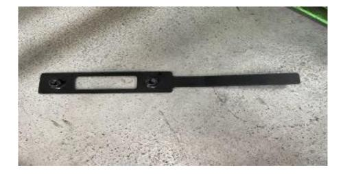
This will need to be held and aligned with the help of a friend or in a way you have access to the side inside of the frame. Use the supplied hardware to mount the bracket with the screw in the opening of the frame. Only finger tighten the bolts & do not fully torque them down just yet.
