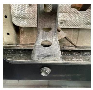
**6.** Once that's done, you can start bolting up the front of the slider with the provided hardware. Please keep in mind that the flat plate with the welded nut on is going to be on the inner inside of the frame. For the front of the slider, you will need the long hardware bracket with 2 nuts welded to it.
